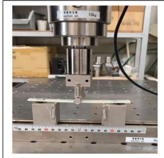
Figure 8: Symbolic 3-Point bending test at Shimadzu AGS-X series test device
