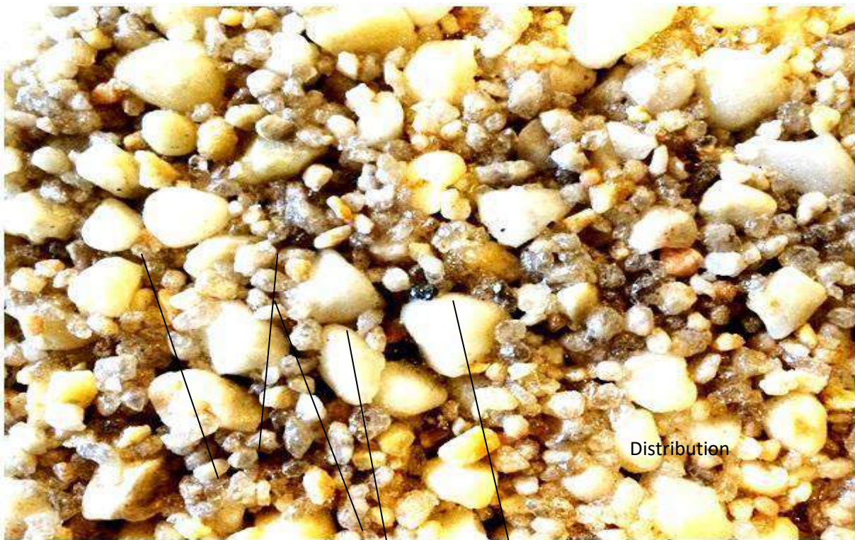
Figure 2. Line Size Distribution Analysis of Sand Specimen for Precision of Image Analysis with comparison of laboratory screen test
