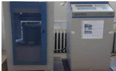
Figure 4 Automatic loading speed controlled press
